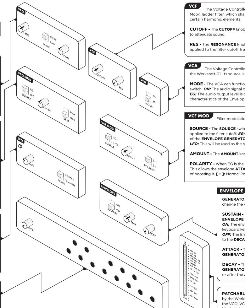
The Voltage Controlled Filter (VCF) is a classic 24dB per octave Moog ladder filter, which shapes sound by attenuating and/or emphasizing certain harmonic elements.
