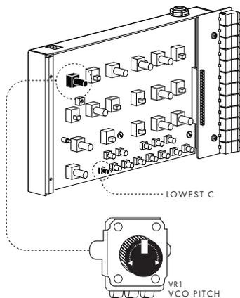
**NOTE:** If it's not obvious what 0 volts is on your CV source, a good way to figure it out is to send notes from your CV source while gently turning VR5 on your Werkstatt. You should hear the Werkstatt's pitch moving up and down as you turn VR5. When you reach a note on your CV source with which turning VR5 no longer produces an audible change in Werkstatt, you have found 0V. Typically this will be a C note on your CV source.
