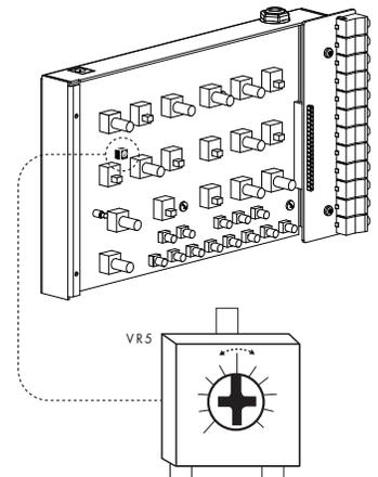
**NOTE:** The final position for VR5 will be somewhere near the center of its travel (and not at either extreme). Turning VR5 past it's stopping point can damage the component and hinder calibration.
