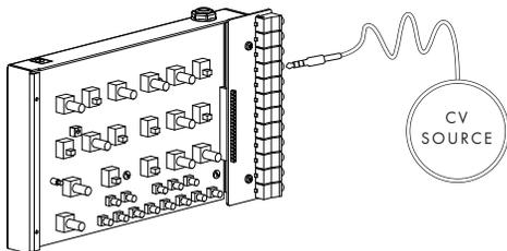
**4** Press the lowest C on the Werkstatt's keyboard, then send 0V from your CV source and use the **VR1 VCO PITCH** knob to tune to a C using a tuner, or tune by ear to match a well calibrated reference instrument that is also driven by your CV source.
