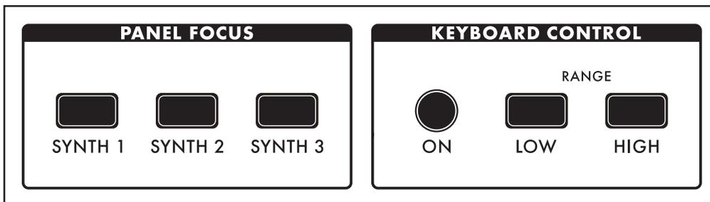
The active Synth is selected using the **SYNTH 1**, **2** and **3** buttons in the Panel Focus module, which allows the Front Panel knobs and buttons to only affect the currently selected Synth(s). Pressing any **SYNTH** button by itself will select just that one Synth. Holding one **SYNTH** button while pressing additional **SYNTH** buttons will select multiple Synths, and allow any tweaks or edits to be applied to all of the selected Synths simultaneously.
