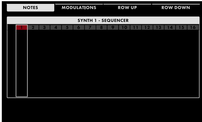
the Master Encoder to scroll left/right through the steps. Two soft buttons at the top of the screen allow you to move the selection Up or Down between rows (Lanes). You can also navigate up and down by turning the Master Encoder while **SHIFT** is active.
