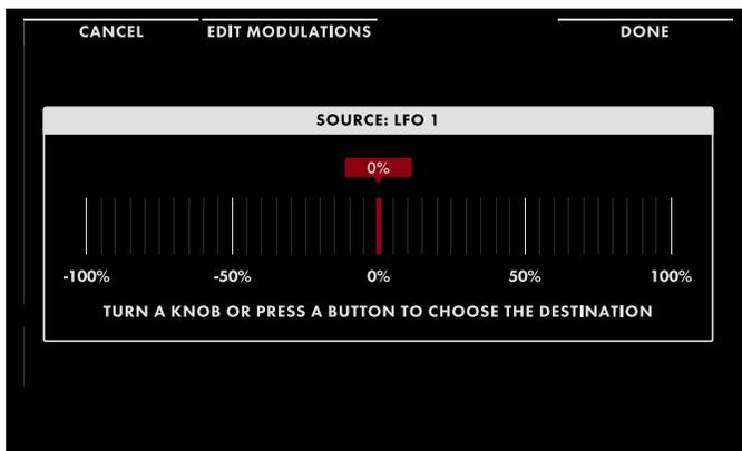
The next Front Panel parameter that is touched or tweaked will become the modulation destination. In this example, the Oscillator 2 **FREQUENCY** knob has been selected, and turning the knob will set the modulation amount as shown in the second screen.
