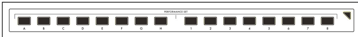
To assign the active Preset to the currently loaded Performance Set, simply press the Bank (A - H) button of your choice, then press and hold the desired Preset (1 - 8) button for 1 second. The Preset button will blink rapidly to let you know your Preset is now assigned to that location.
