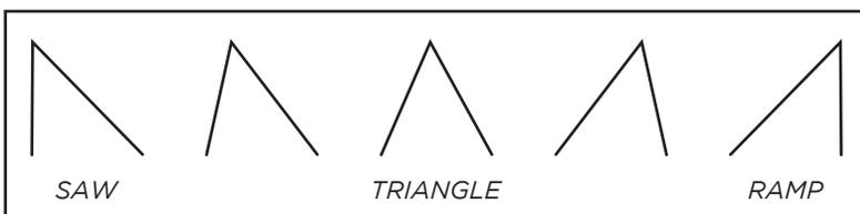
**NOTE:** In **TRI** mode, the rising and falling phases of the wave both scale with pitch -- both get faster at higher pitches, and both get slower at lower pitches.
