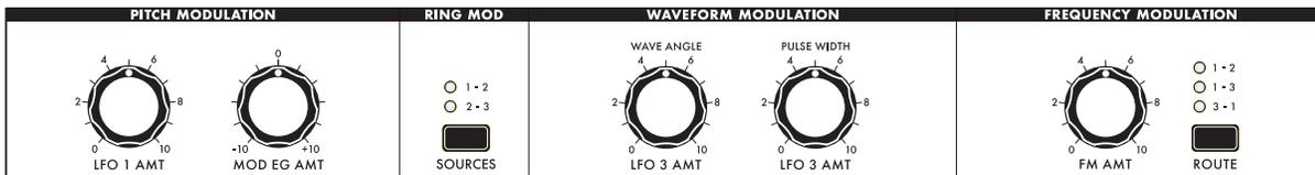
Here, the Pitch Modulation and Waveform Modulation parameters are applied to all Oscillators equally. Selecting the Ring Modulation sources and choosing a Frequency Modulation routing are also performed using the controls found in this section.
