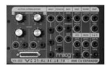
The VX-352 (exclusively for the RME) contains all of the Voyager *inputs* on ¼" jacks (13 CV inputs and 5 Gate inputs), along with two active attenuators with offset and one 4-way multiple. Both the VX-351 and VX-352 connect to the Voyager's accessory ports with a supplied DB-25 style cable.
