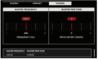
**MASTER FREQUENCY** (400 Hz to 480 Hz) This parameter controls the base frequency for equal-tempered tuning of the Moog One. This is the reference point for "concert pitch," defined as the frequency of the A note above Middle C (MIDI Note # 69). The default value is 440 Hz.
