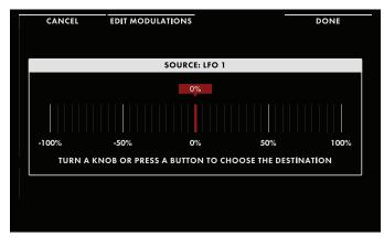
The next Front Panel parameter that is touched or tweaked will become the modulation destination. In this example, the Oscillator 2 **FREQUENCY** knob has been selected, and turning the knob will set the modulation amount as shown in the second screen.
