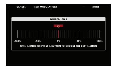
The destination will be assigned automatically to the first hardware parameter that is touched or operated. In this example, Oscillator 2 Frequency has been chosen as the modulation destination. As the destination parameter knob is turned, the value in the display will change to show the depth of the modulation effect being applied.
