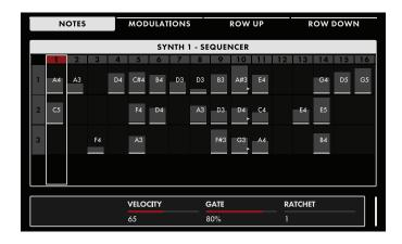
Each lane can only support one note per step, so adding more lanes is required to have multiple notes on each step. Pressing the ROW DOWN Soft button is one way to add an additional lane. You can also simply play multiple notes on a single step; Moog One will create a new lane for each additional note played. Only one lane can be active/highlighted at once, so if you create an additional lane and play only a single note for that step, it will be entered into the active lane.
