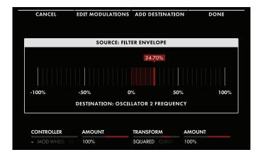
In this example, the Oscillator 2 **FREQUENCY** knob has been selected, and turning the knob will set the modulation amount as shown in the second screen. At this point, pressing the DONE Soft Button at the top of the screen will complete the modulation routing, or the CANCEL Soft Button can be used to exit this modulation screen without making the modulation route complete. The functions of the additional Soft Knobs and Soft Buttons are discussed in the MODULATION section.
