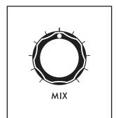
The balance between the two Filter outputs is controlled using the **MIX** knob. The center position represents an equal blend of the two filter modules. Turning the **MIX** knob to the left will favor the SVF output; turning the **MIX** knob to the right will accentuate the Ladder Filter output.
