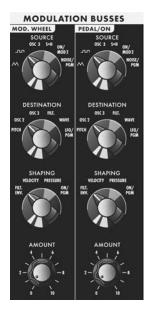
The Modulation Busses allow you to select a variety of modulation sources, destinations, modulation shaping, and amounts. The two Mod Busses are labeled MOD WHEEL and PEDAL/ON. The performance control for the MOD WHEEL Buss is the Modulation Wheel itself, while the performance control for the PEDAL/ON Buss is the MOD I Input jack on the Patch Panel.
