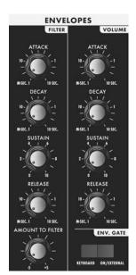
When triggered, EG's produce a time-varying control voltage that has a specific start, middle and end profile. The parameters that define this CV profile are Attack, Decay, Sustain and Release, sometimes abbreviated as ADSR.
