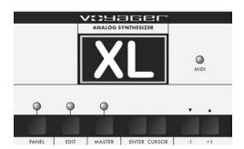
The status display is an LCD screen located within the Interface Panel. When the Voyager XL is first powered on, the screen will display an 'XL' greeting message. The message will stay on the screen for a few seconds, and then the screen will display the active preset. This preset will be the last preset in use when the Voyager was powered down.
