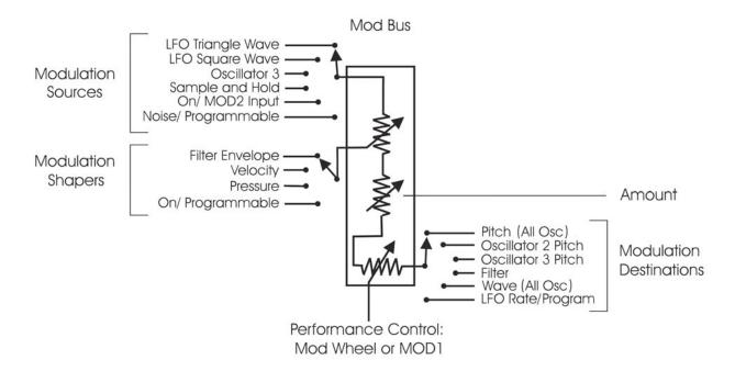
Three controls modify the amount of modulation: the **AMOUNT** control, the **SHAPING** control, and the Mod Wheel (for the Mod Wheel Mod Buss) or MOD1 level (for the Pedal/On Mod Buss). The **AMOUNT** control sets how much both the Mod Wheel/MOD1 Input and the Shaping CV allow the mod source through to the mod destination.
